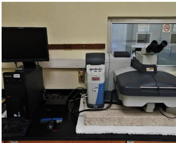
**Figura. 27. Microscopio DXR3 micro-Raman Thermo Fisher Scientific.**
