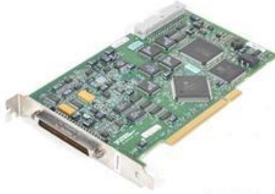
**Figura 4.24** Tarjeta PCI6024E National Instrument.
