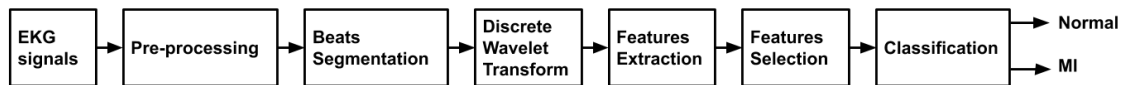
Figure 1.3: Block diagram of the Acharya's method for classifying MI, from Acharya et al. [9].
